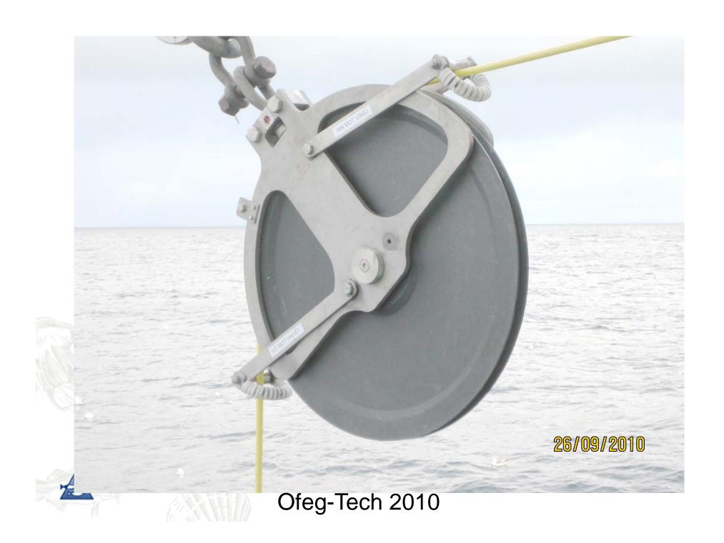
Strain relief with integrated counterpart for the latch
